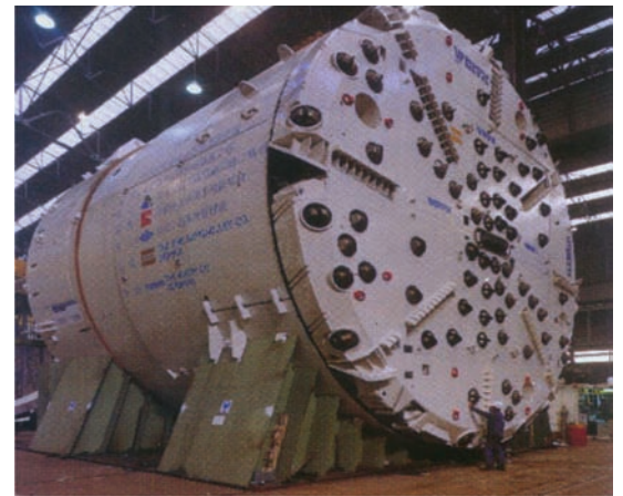
雪山隧道主坑 TBM
