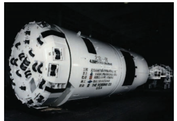
雪山隧道導坑 TBM
